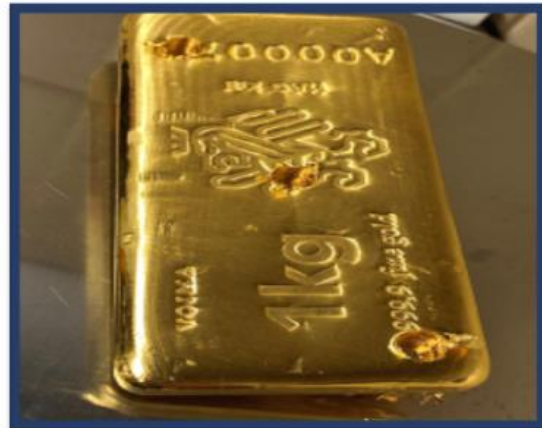
12) Bar after being drilled/sampled.
