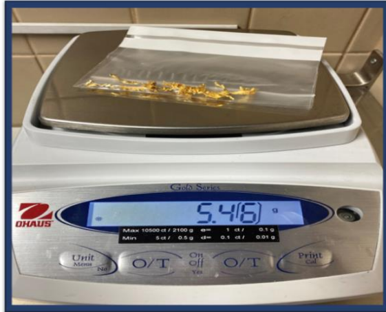
13) Drilled sample material being weighed
