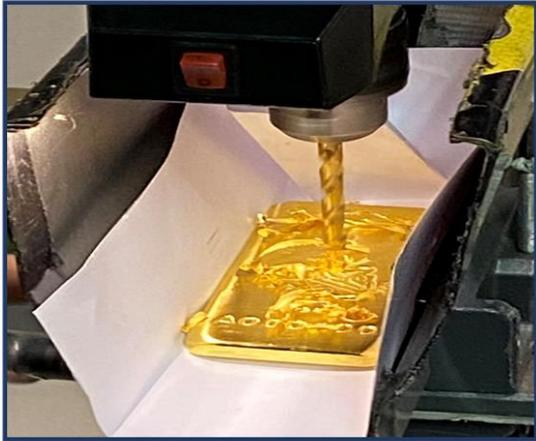
9) A 1000 gram bar being drilled/sampled.
