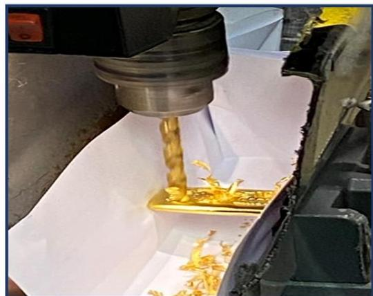
8) A 100gram bar being drilled/sampled
