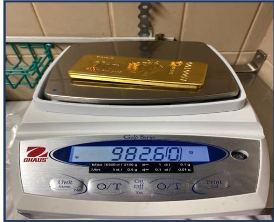
10) A sampled/drilled bar being check weighed
