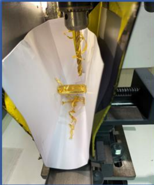
11) Bar being drilled/sampled.
