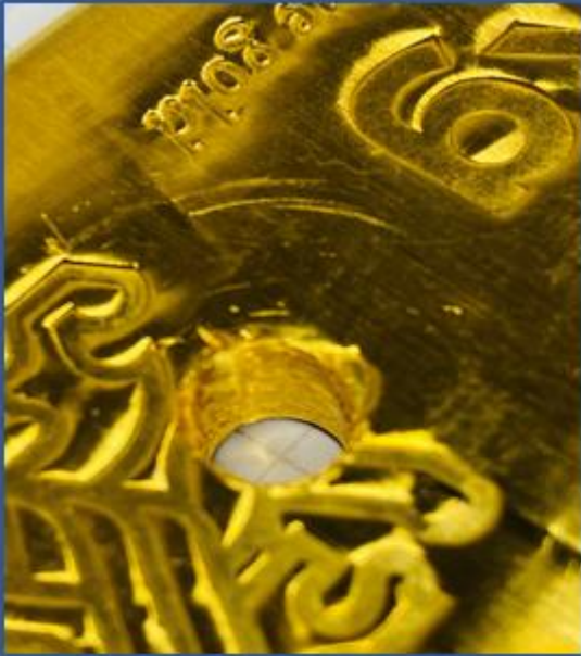
13) Bar being drilled/sampled.
