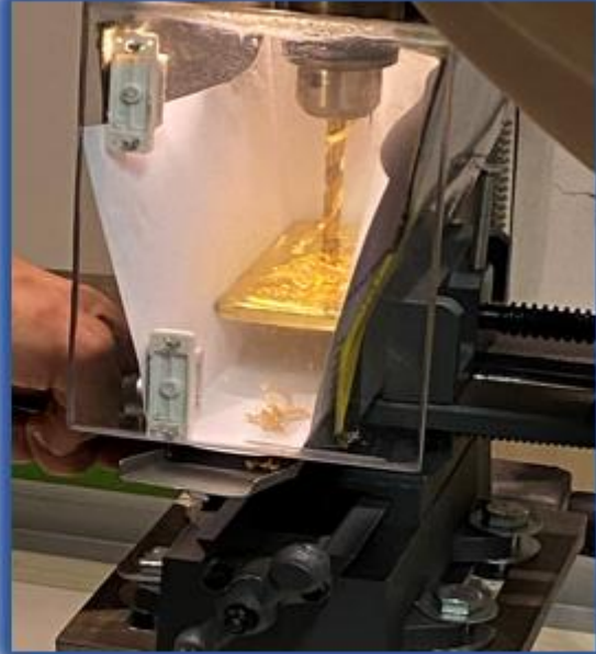
10) Bar being drilled/sampled.
