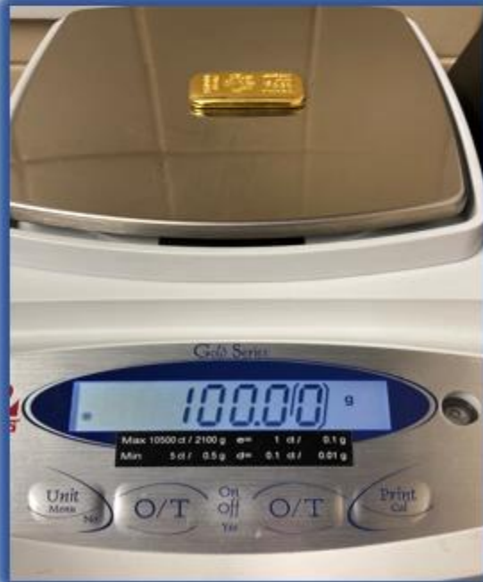
8) Bars being check weighed.
