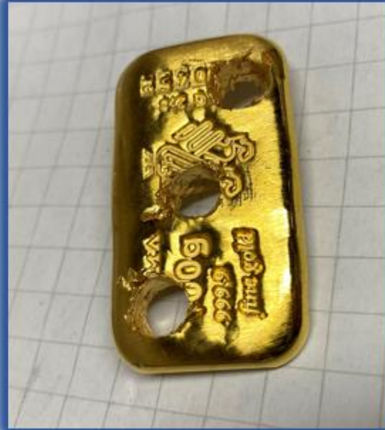
14) Bar being drilled/sampled.
